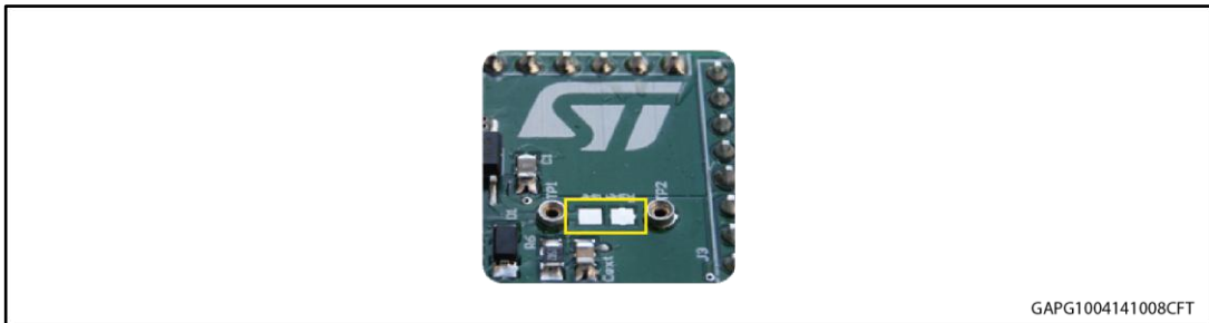
Figure 5: Pads for soldering SMD resistor
