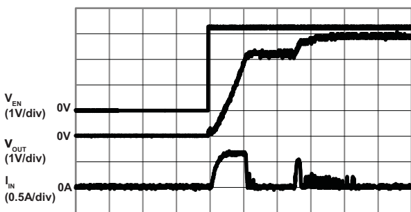
Soft Start ( V_{\text{OUT}} = 3.8\text{V} ; V_{\text{IN}} = 3.3\text{V} ; I_{\text{OUT}} = 0\text{A} )
